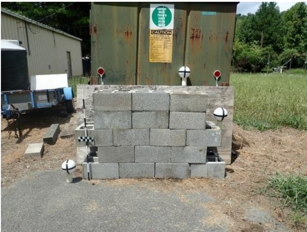
Figure 12: Double-layer brick wall simulating a creek bank surface
