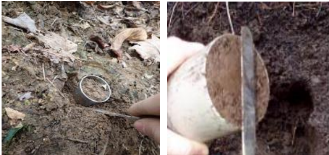
Figure 17: (a) the soil around the core was removed, then (b) the excess soil from the bottom was detached from the cylinder's surface.
