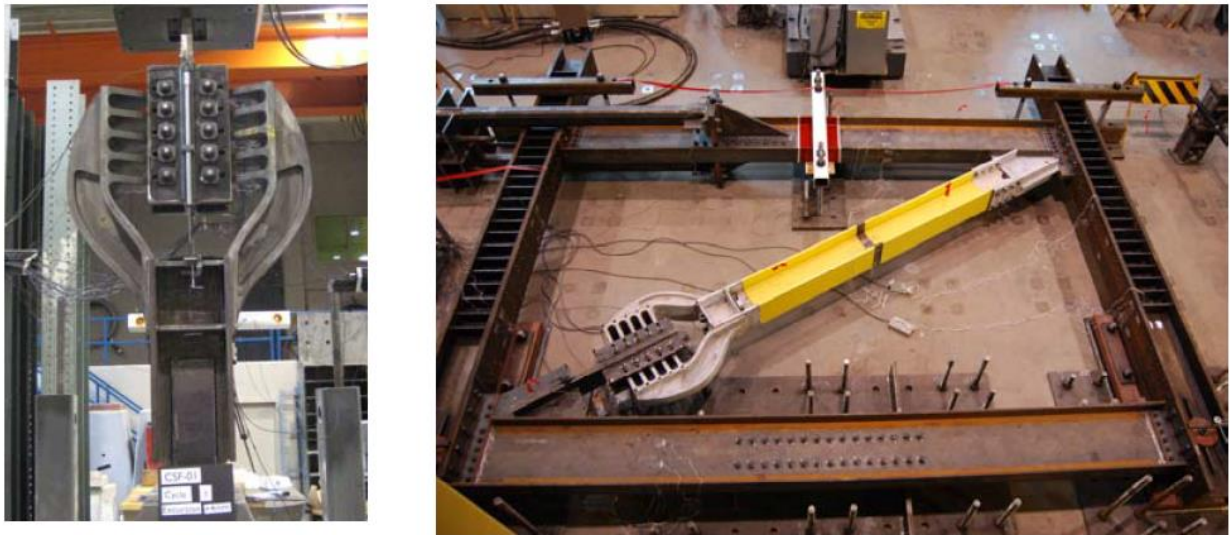
Figure 7. YBS prototype. YBS component (left) and full scale frame (right).
