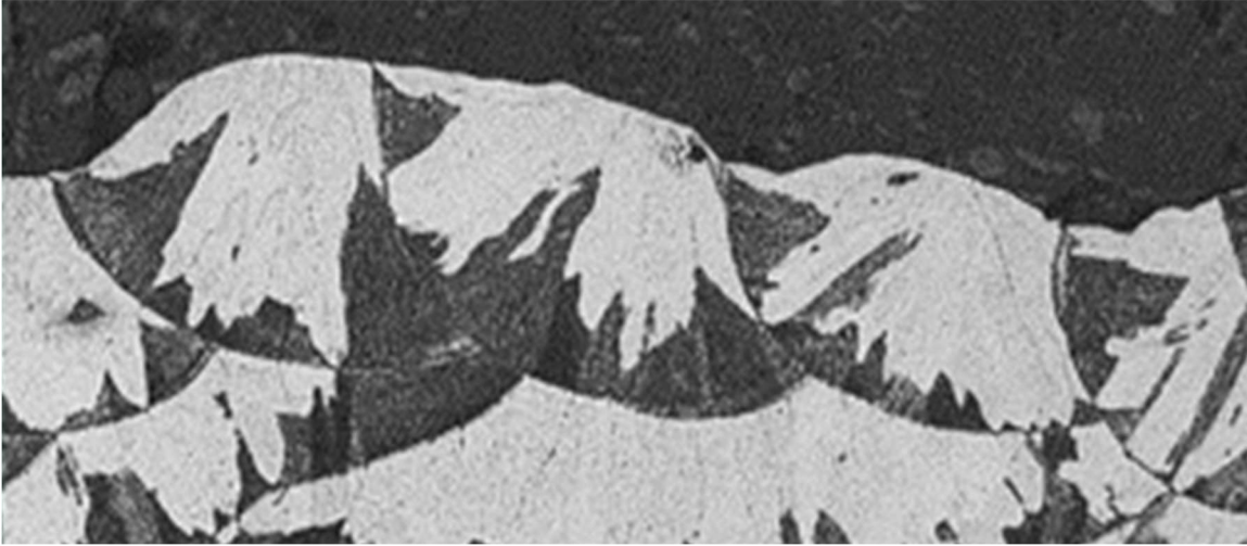
Figure 6: Etched optical micrograph of sample 6 of the parameter study build revealing stark etching contrast. Ref: Unpublished research by Simpson et al.
