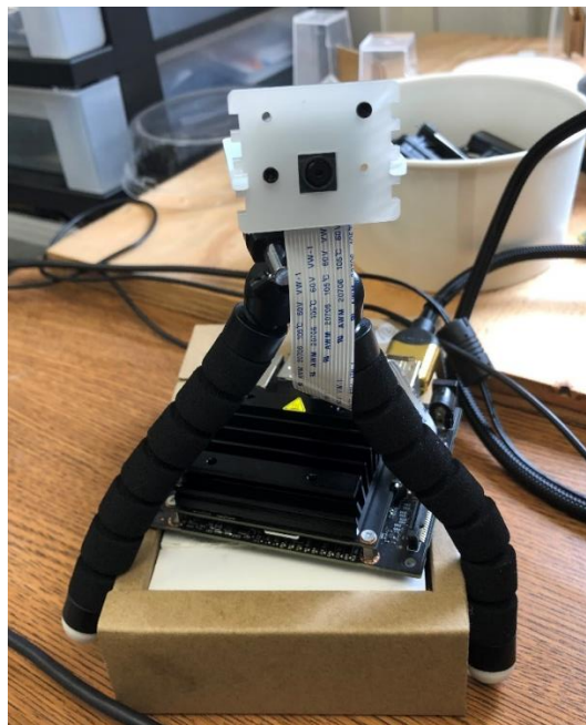
Figure 4.2 shows the Jetson Nano system. It includes a mini tripod and custom camera holder to keep the camera pointing straight.
