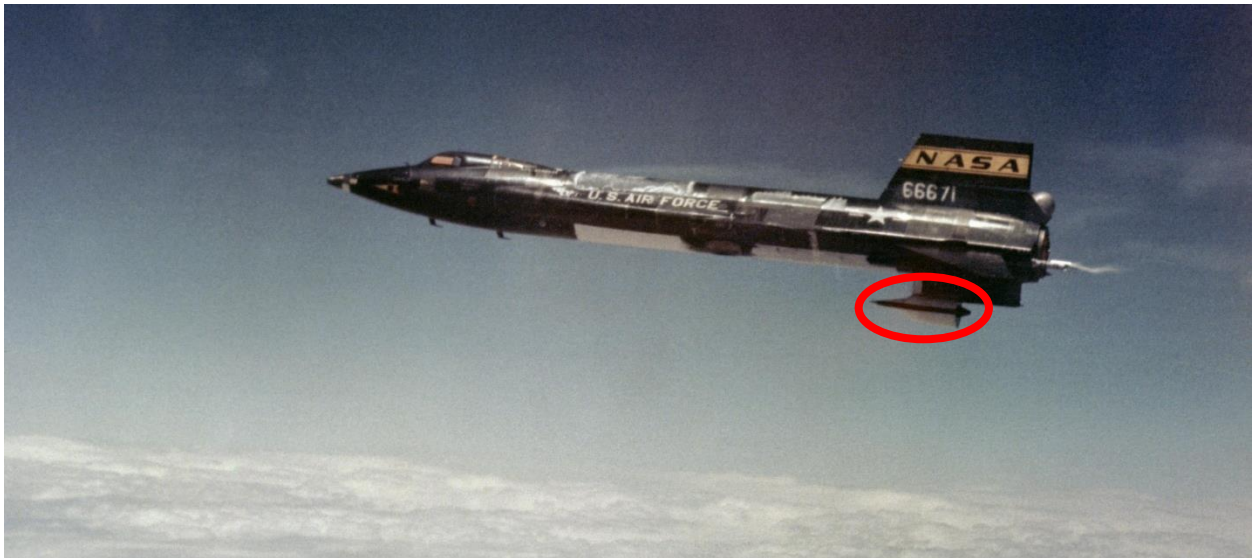
Figure 1.1. Photograph of the X-15A-2 with the dummy ramjet (circled) attached. Image courtesy of NASA, 1967.
