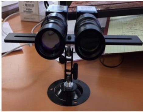
Figure 2.2 (a) Two CCD cameras mounted with the band-pass filters (460-nm and 520-nm filters); (b) Experimental setup in an indoor lab with ambient light.
