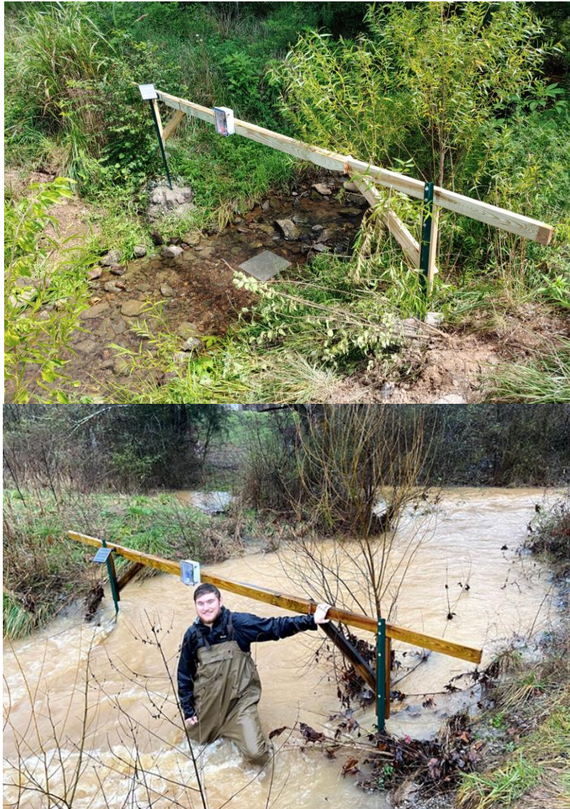
Figure 2.2. Stream gauging station installed at the upstream site during baseflow (top) and flooding (bottom) conditions.
