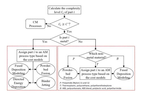
Figure 2.1 AM process selection framework.
