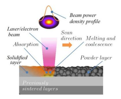
Figure 1.4 Schematic view of SLS/SLM (Lawrence, 2014).
