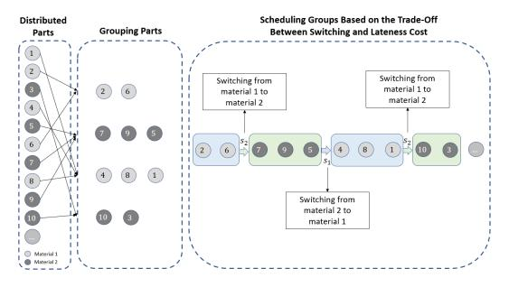
Figure 4.1 Demonstration of the proposed scheduling model
