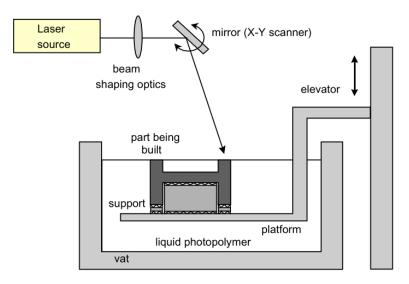
Figure 1.2 A schematic view of the stereolithography (Park et al., 1998)
