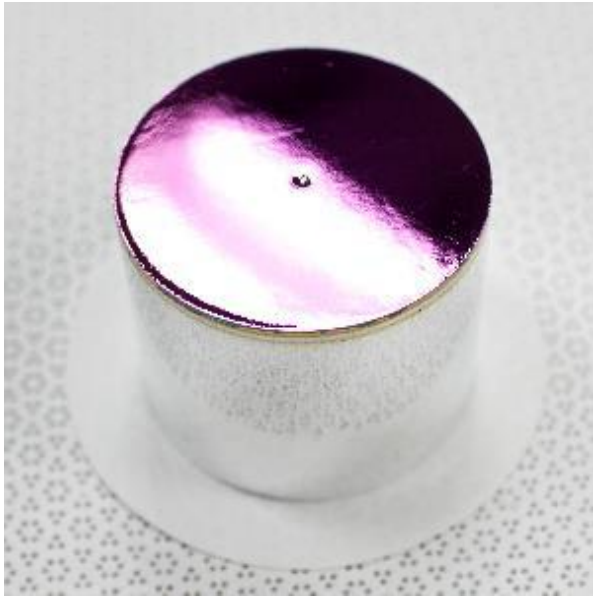
Figure 3.3: Image of a MAJORANA high purity germanium PPC crystal (left) and a MAJORANA detector unit with attached electronics front end board (right).
