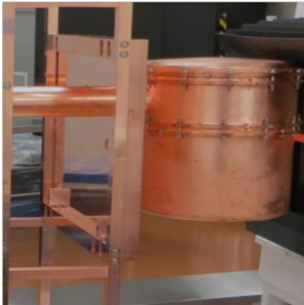
Figure 3.2: Cryostat of one module during insertion into the shield (left) and during detector string installation (right).
