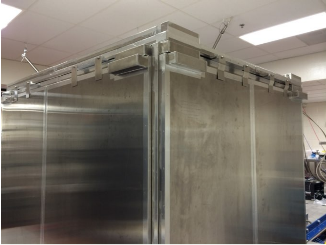
Figure 4.1: Veto Panels in place on MJD
