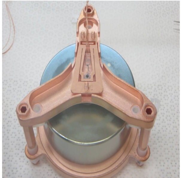
Figure 3.3: Image of a MAJORANA high purity germanium PPC crystal (left) and a MAJORANA detector unit with attached electronics front end board (right).
