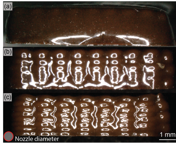
Figure A.2: Optical micrographs of the as-printed ends of representative epoxy/FS longitudinal rectangular bars: (a) contains 5 wt.% FS, (b) contains 7.5 wt.% FS, and (c) contains 10 wt.% FS.
