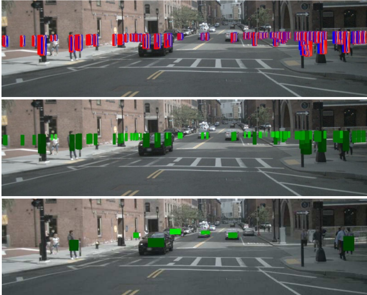
Figure 5.4: Expanding radar points to 3D pillars (top image). Directly mapping the pillars to the image and replacing with radar depth information results in poor association with objects' center and many overlapping depth values (middle image). Frustum association accurately maps the radar detections to the center of objects and minimizes overlapping (bottom image). Radar detections are only associated to objects with a valid ground truth or detection box, and only if all or part of the radar detection pillar is inside the box. Frustum association also prevents associating radar detections caused by background objects such as buildings to foreground objects, as seen in the case of pedestrians on the right hand side of the image.
