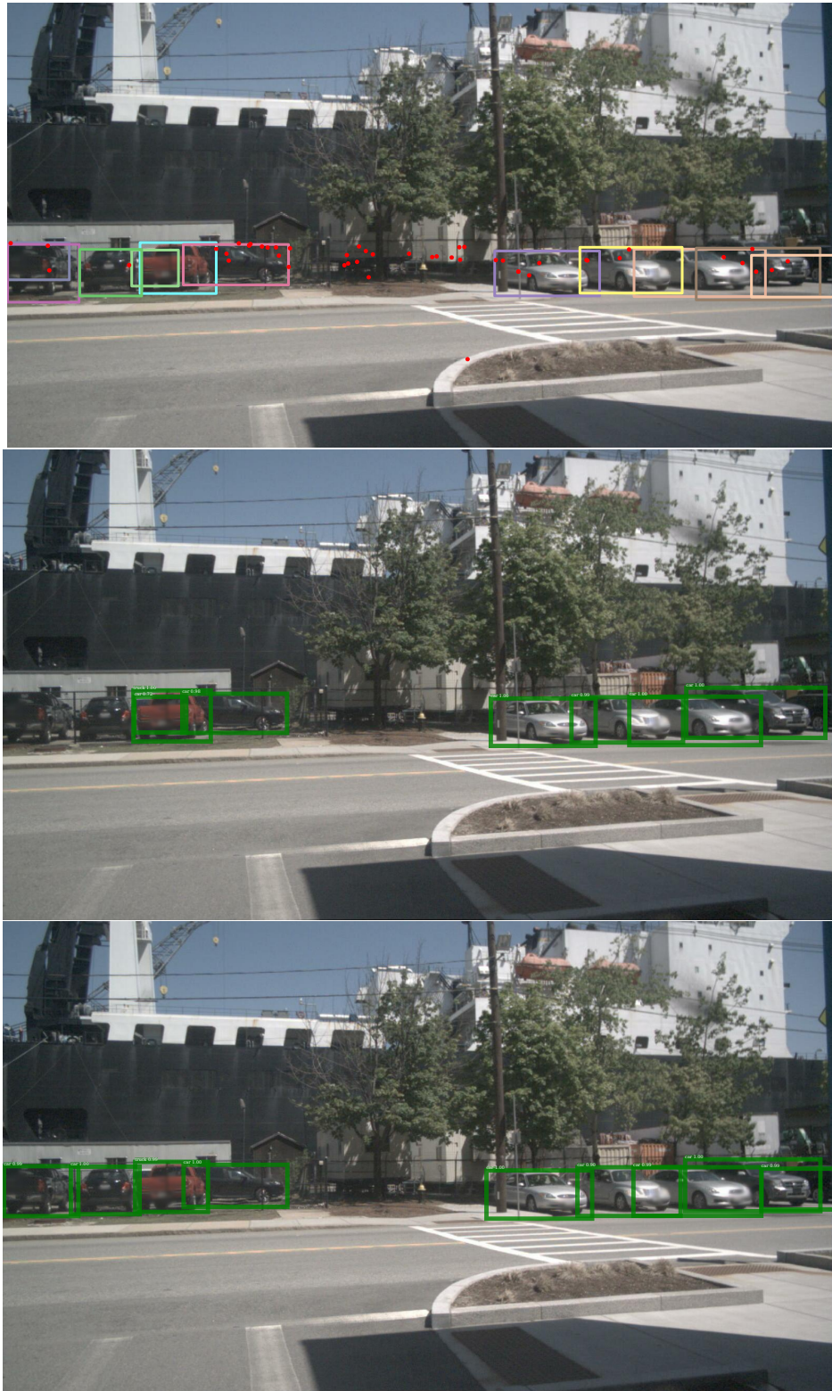
Figure 3.3: Detection results, cont. Top row: ground truth, middle row: Selective Search, bottom row: RRPN
