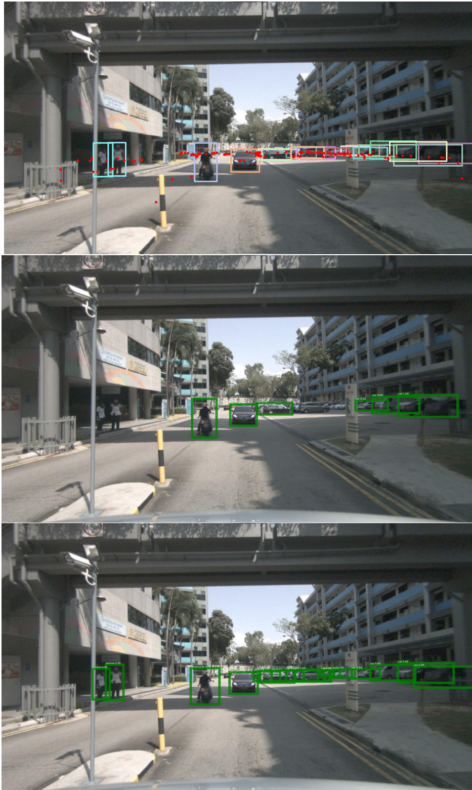
Figure 3.5: Detection results, cont. Top row: ground truth, middle row: Selective Search, bottom row: RRPN
