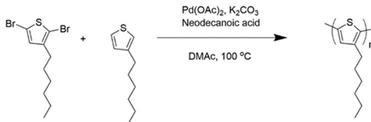
Figure 3.6: Optimized DArP conditions used to synthesize poly(3-hexylthiophene) as a test reaction.
