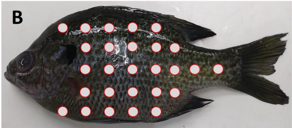
Figure 24. Relative durometer measurement locations (circles) were taken on the left side of (A) Gelfish cast without skin and (B) bluegill with scales. Durometer measurements were replicated for both Gelfish and actual bluegill, i.e., n = 3 for each. The Gelfish models and bluegill were \sim 16 cm total length and \sim 90 g mass. We also measured Gelfish with surrogate skin and bluegill without scales at the same approximate locations (not pictured).
