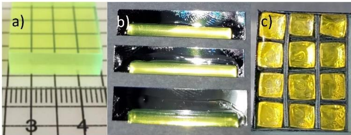
Figure 8.3. Images of a) the BiPVT source sample (6.85 × 19 × 21 mm) provided by LLNL, b) the individual BiPVT pixels, adhered to ESR, prior to trimming, and c) the final BiPVT 4×3-pixel array face, which is placed in contact with the Varex radiographic panel.
