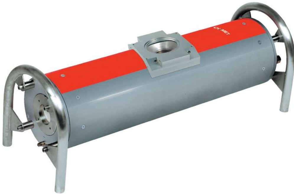
Figure 5.7. Image of the Comet MXR-451/26. This RGD contains a bipolar oil-cooled x-ray tube with a tungsten anode and 5mm of beryllium beam shielding. It is designed specifically for NDA.
