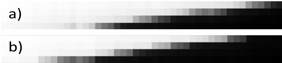
Figure 9.5. Measured composite 4x45-pixel images of a 6.35 mm-thick steel phantom edge for a) EJ-256 and b) EJ-200. These images were constructed from 15 separate measurements at varying degrees of array shielding, with the phantom edge offset from the pixel alignment at a 5° angle.
