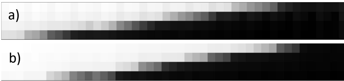
Figure 7.1. Image of initial, 4x45-pixel, composite images for a) BiPVT and b) EJ-200 measured in the 370 kVp x-ray environment.
