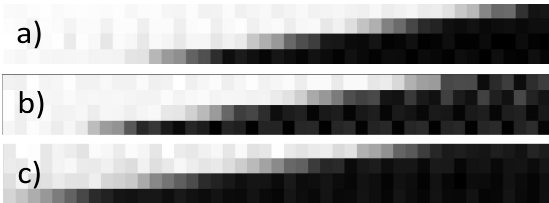
Figure 9.7. Simulated composite 4×45-pixel images of the 6.35 mm-thick steel phantom steel edge for a) EJ-256, b) EJ-200, and c) BiPVT. These images were assembled from 15 separate combined simulations of both MCNP6 and OpticStudio, each with varying degrees of array shielding, with the phantom edge offset at a 5° angle from the pixel alignment.
