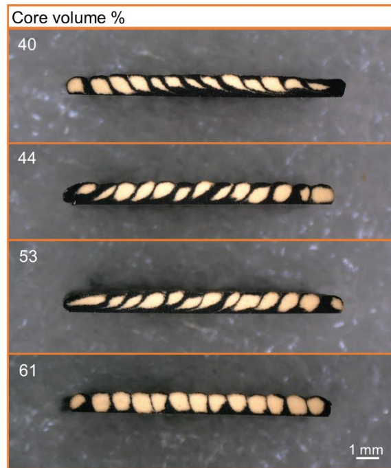
Figure 3.15. Optical micrographs of C-S cross-sections printed with S32HS foam.
