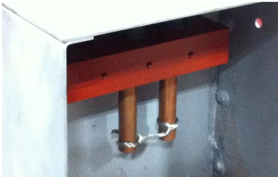
Figure 21 - Close-up Showing Fuse Wire for Test Run #1
