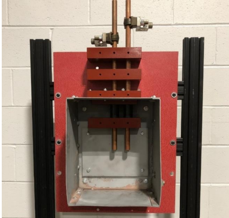
Figure 16 - Single-phase Arc Flash Test Fixture
