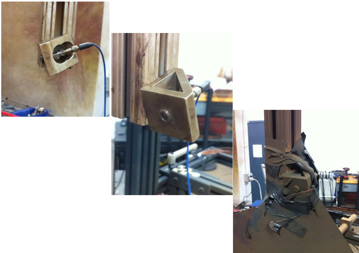
Figure 19 - Blast Pressure Sensor Mounting and Cable Protection
