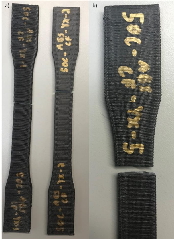
Figure 54 a) Different break locations on specimens. b) typical break pattern.
