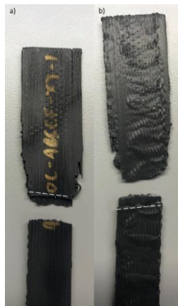
Figure 52 a-b) Multi-layered failure exhibited by specimen 90C_CF-ABS_XY_1, dashed white lines illustrate layer separation.
