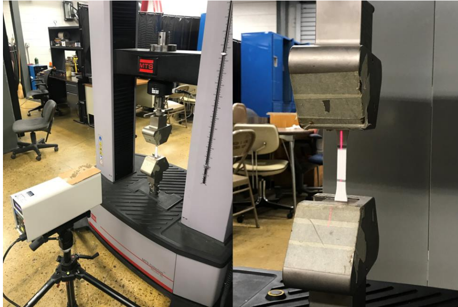
Figure 40 MTS load frame with laser extensometer and specimen loaded with reflective tape attached for extensometer
