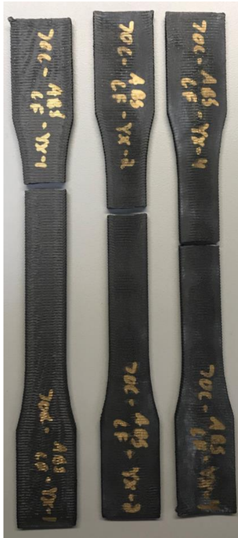
Figure 55 Different break locations on specimens.
