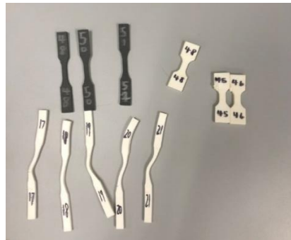
Figure 59 Shape change associated with heating material beyond the T_g where the material expanded in the bead width and contracted in the bead length.
