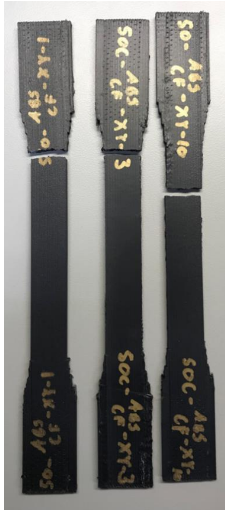
Figure 51 Typical break location of test set (left), outlier specimen (middle), gauge length break (right).
