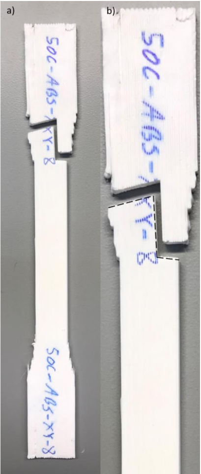
Figure 43 a) Failure in Z shape pattern within the fillet region. b) Highlighted (black dashed line) Z shape failure pattern.
