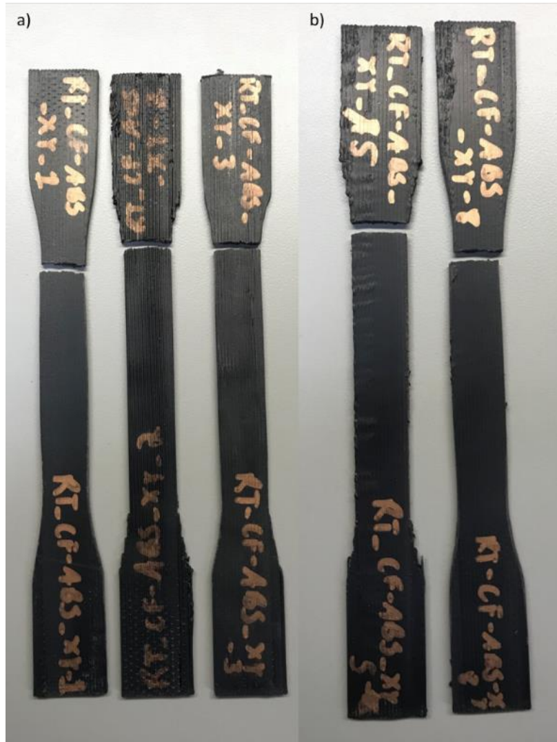
Figure 50 a) Specimens showing the filing, non-filing, and reduced filing. b) Outlier specimens in the test set.
