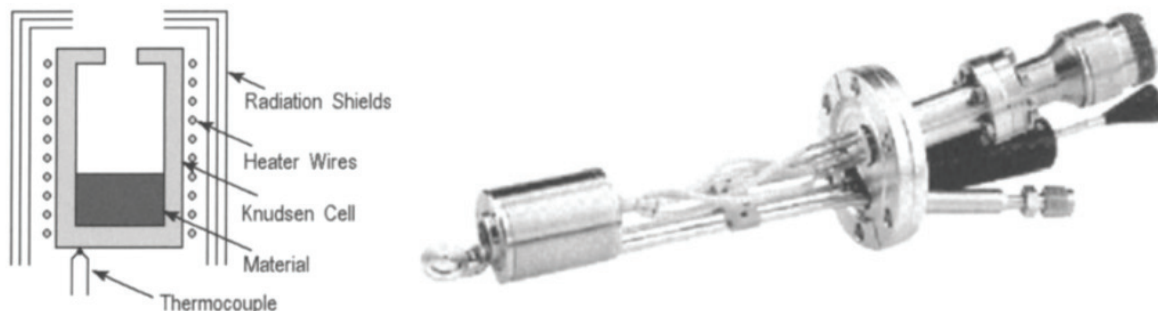
Figure 2.2: left: A schematic diagram of the effusion cell head. right: A SciCam low-temperature effusion cell used for Pb deposition in this work. (Oura et al. , 2010)
