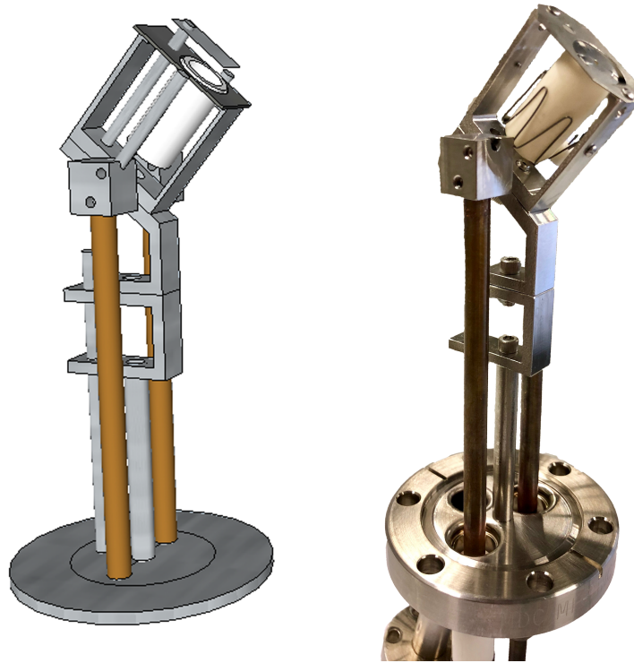
Figure 2.3: left: A drawing of a custom effusion cell designed for deposition onto a sample close to the cold LT-STM location. right: Final configuration of the custom effusion cell with radiation shield and shutter removed.
