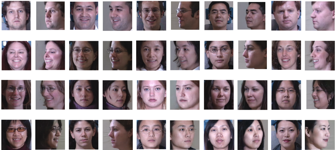
Figure 7.4: Reconstruction of profile images at the output of the profile U-Net generator with frontal images as input to the frontal U-Net generator. Every odd number column represents the input frontal image, and every even number column represents the output profile image. The input images belong to the CMU-MultiPIE dataset.
