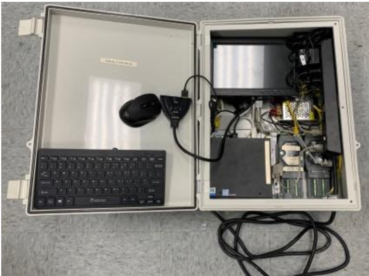
Figure 4. Data Acquisition Box
