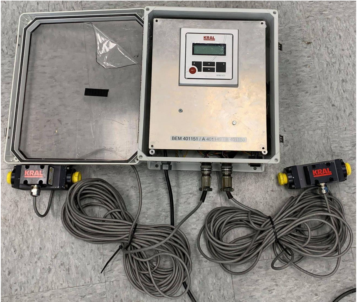
Figure 7. KRAL BEM 500 Display and KRAL OEM 20 Diesel Flow Meters
