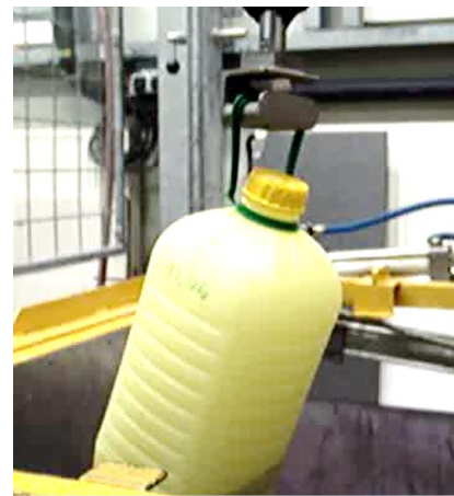
Figure 3. Drop test method for handles resistance.
