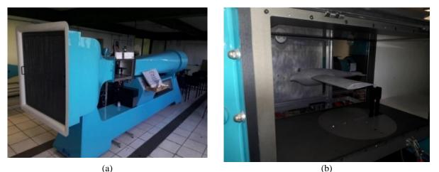
Figure 15. (a) The AeroLab subsonic wind tunnel and (b) the UAV prototype.
