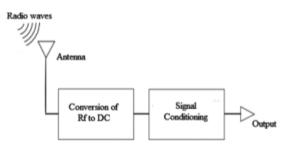
Figure 1. Based energy harvesting system RF [6].
