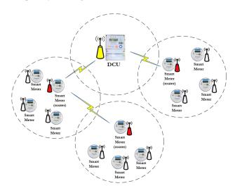
Fig. 2. Advanced metering infrastructure (AMI) network topology.
