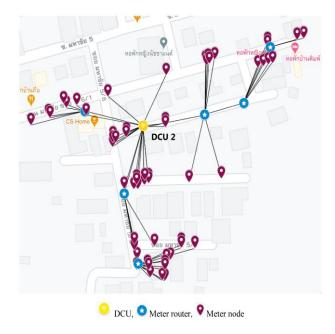
Fig. 10. AMI network topology for DCU location 2 in suburban area, Nakhon Ratchasima City.
