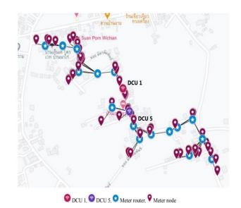
Fig. 12. AMI network topology for 2 DCUs at DCU location 1 and location 5 in the rural area, Nong Khai Province.
