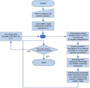
Fig. 3. A flowchart of the proposed optimal DCU placement algorithm.
