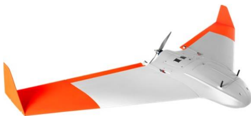
Fig. 5. Drone – Fixed wing (Ai450 v2.5 ER) [25].
