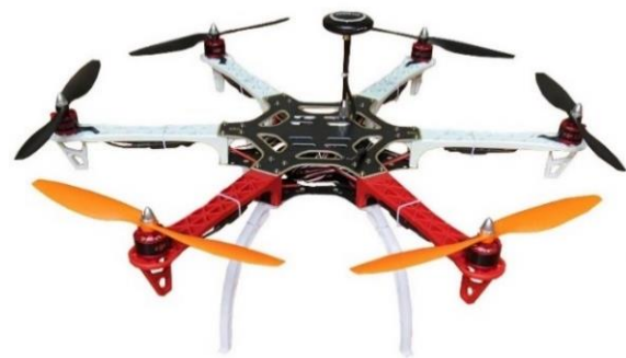
Fig. 3. Drone – Hexacopter (Hobbypower DIY F550 Hexacopter Frame Kit) [17].
