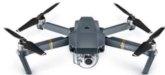
Fig. 2. Drone – Quadrotor (DJI Mavic Pro Platinum) [16].
