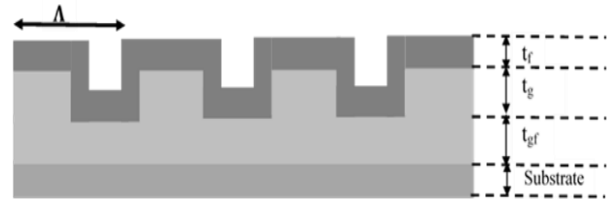
Fig. 2.2 Structure of GMR simulated in RCWA.
