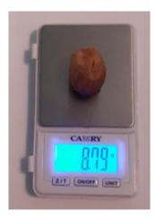
Fig. 10. Camry scale used for measuring date fruit mass.
