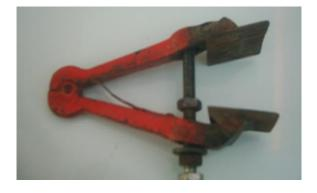
Fig. 3. Clamp for holding the date bunch during shaking.
