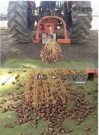
Fig. 1. Tractor-mounted bunch shaker [29].
