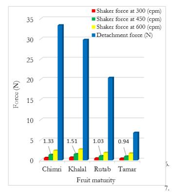
Fig. 13. The fruit detachment force and the dynamic shaker force for Zahdi dates at subsequent maturity.
