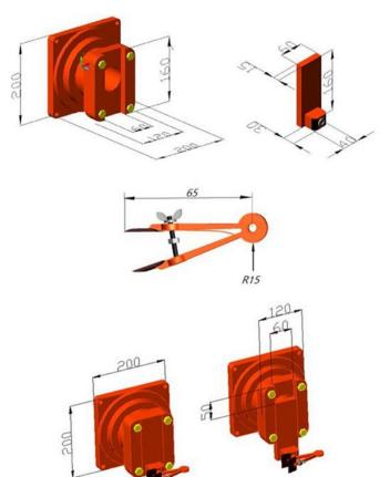
Fig. 7. CAD Modeling of bunch shaker.
