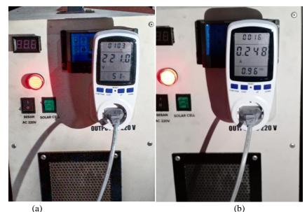
Figure 5: Fan loading (a) Measurement of alternating output voltage (b) Measurement of alternating current when loading fan
