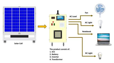
Figure 1. Schematic of the battery charging device
