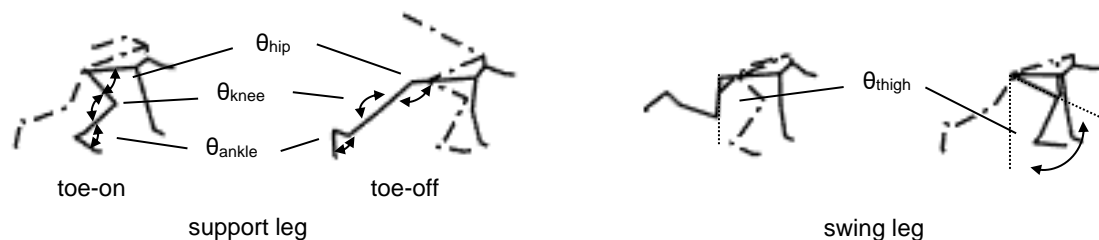
Figure 1: Definition of the joint and segment angles for the right leg.
