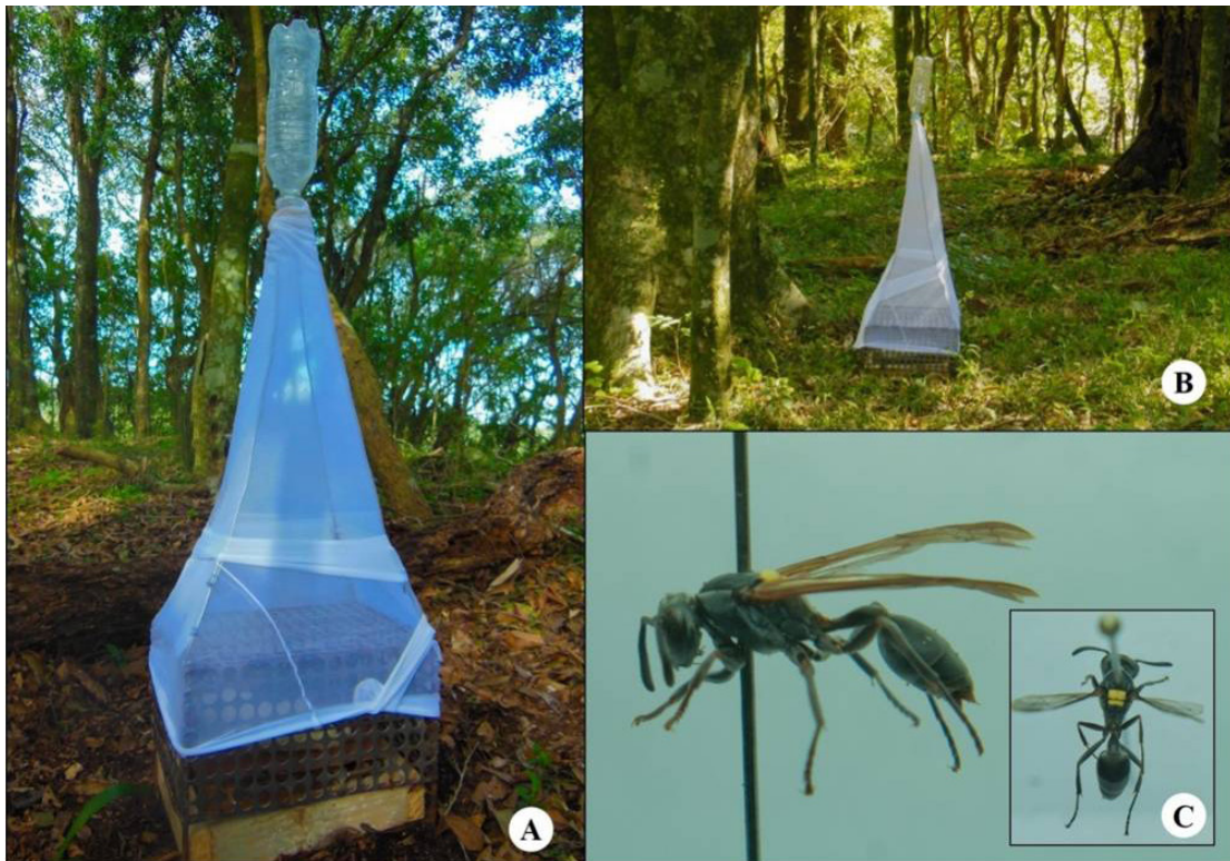
Fig 1. A – Shannon trap containing PET bottle of 500 ml, nylon pyramid, iron cage and wooden tray; B – Trap in the forest area; C – Lateral and dorsal view of Polybia scutellaris .
