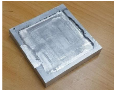
Figure 4.2 Aluminium socket for housing mica heating pad for the laboratory thermal tests
