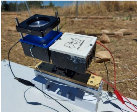
Figure 4.13 Outdoor setup of the 11.2x11.2 and 62x62 TE modules
