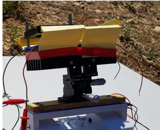
Figure 3.15 Cardboard sheets to reduce wind influence on the module
