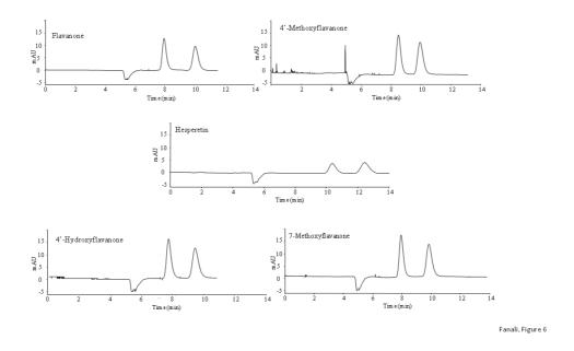
Figure 7 - Enantioseparation of selected flavanones analyzed by CEC employing a capillary column packed with SM- $\beta$ -CD (A) MeOH/H<sub>2</sub>O, 5 mM ammonium acetate pH
