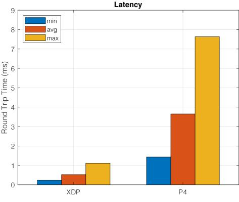
Figure 5. Latency of XDP vs. P4.
