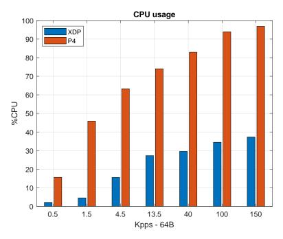
Figure 7. CPU consumption of XDP vs. P4.
