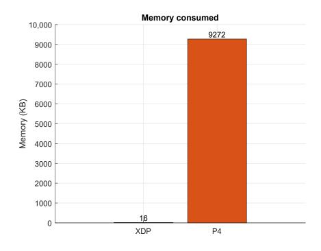
Figure 6. Memory consumption without shared objects of XDP vs. P4.
