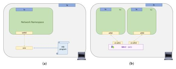
**Figure 1.** Example of the developed wired scenarios: (a) XDP wired scenario (left); (b) P4 wired scenario (right).
