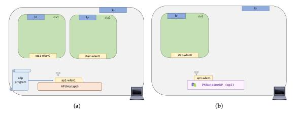
**Figure 2.** Example of the developed wireless scenarios: (**a**) XDP wireless scenario (**left**); (**b**) P4 wireless scenario (**right**).
