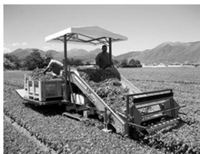
Fig.2 FR32 harvester with a kit for harvesting medicinal plants
