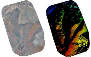
Figure 5: Orthomosaic and the corresponding sparse Digital Surface Model (DSM) before sensification derived from drone-based images using Postflight Terra 3D powered by PIX4D in Mintia area, Hunedoara county.
