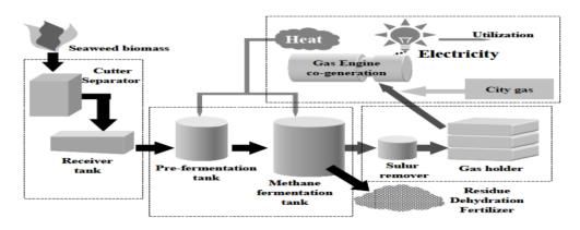
Figure 2. Seaweed processing plant for production of methane and electricity (Matsui et al., 2006)
