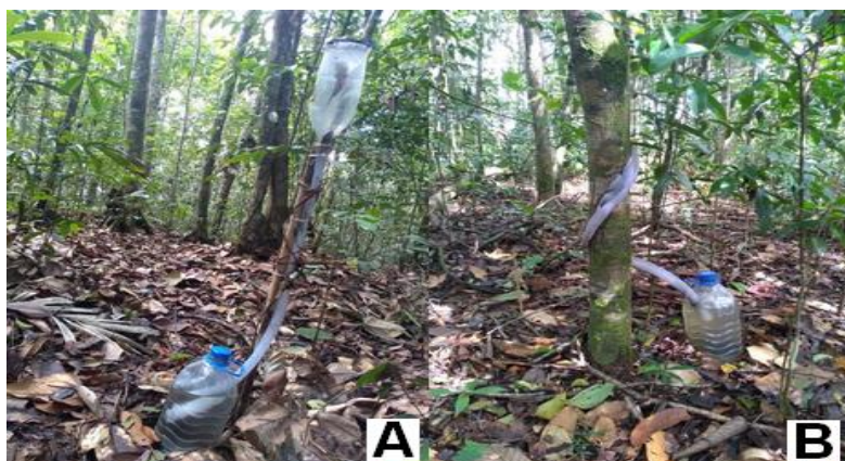
Figure 3. Collector system used to capture rainfall (a) and stemflow (b) of forest species in the fragment of the Dense Ombrophilous Forest of the Lowlands, in Sirinhaém, Pernambuco, Brazil.
