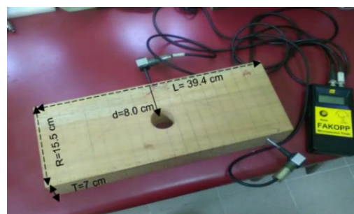
Figure 2. Block 1 with a 2.5 cm diameter cavity, layout of the 23 kHz Micro Timer ultrasound equipment.
