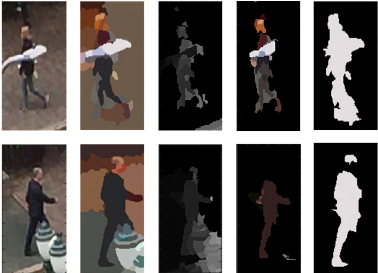
Figure 11: Examples of the results obtained with partial occlusion. Pedestrian hidden by a lamp (row 1) or pole (row2). From left to right: input images, the initial segmentation, the classification by clustering, the probabilistic relaxation, and the ground truth.
