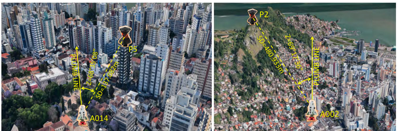
Figure 7: Real examples of surveys with zenith angles away from the horizon for geodetic networks in urban areas.
