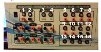
**Figure 2**. Test stand for electronic vehicle control unit with electronic injection systems. [9].
