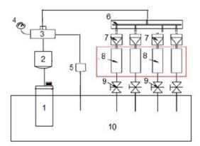
Figure 7. Hydraulic system: 1) gasoline pump, 2) filter, 3) teee,4) manometer 5) return, 6) rail, 7) injectors, 8) measuring pipes, 9) solenoid valves, 10) tank. Source: own.
