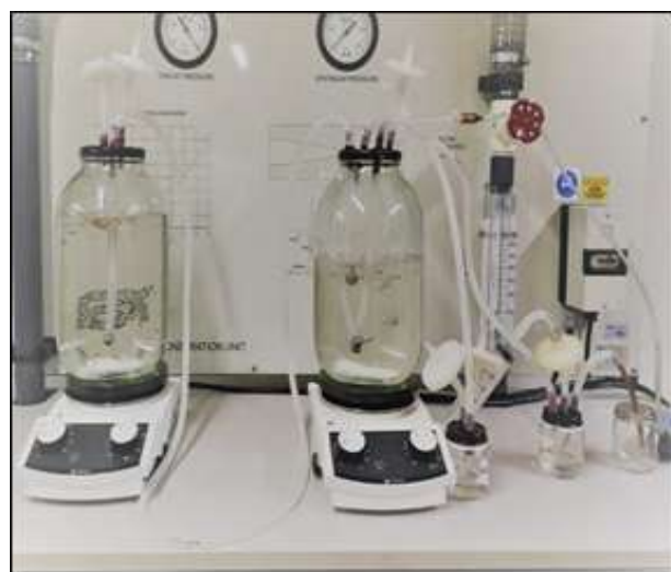
Figure 2. Pilot fermentation system designed for the alcoholic fermentation process. Source: own.
