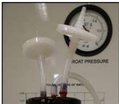
Figure 4. Hydrolysis Content System Filters “in house”. Source: own
