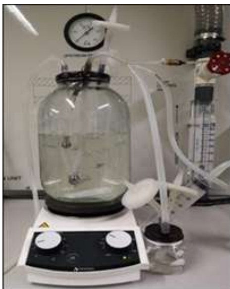
Figure 8. Pilot fermentation system. Source: own
