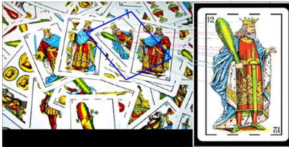
Figure 7. Recognition of objects with occlusion. Source: own.
