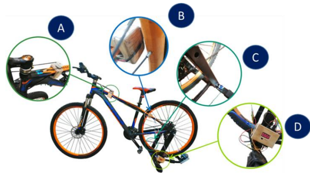
Figure 2. Implemented system for capturing kinematics variables in a conventional bicycle during static operation. Coupling systems details and elements used are shown (A: Turning angle system, B: Hall effect sensor, C: Servomotor, D: Arduino with display)
