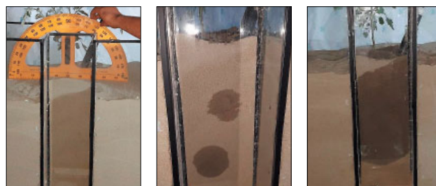
Fig. 4. The pile method for studying the water distribution boundaries: a – determining the peg angle when installed at an angle; b – initial soil moisture; c – complete soil moistening
