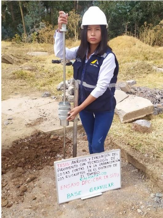
**Figura 12:** DCP in situ – base granular
