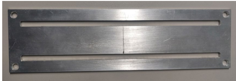
Figure 5.2: Machined Sensor substrate
