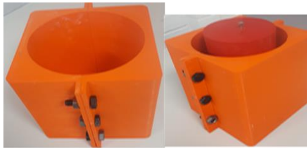
Figure 1: 3D Pictures of assembled wax moulder for (a) Solid, (b) hollow shape [29]
