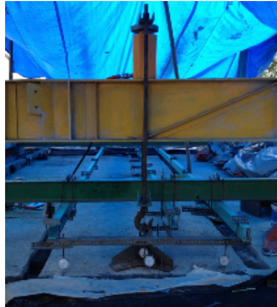
Fig. 3 Photographs of pull out loading tests on 1 pile row full scale Nailed-slab [1].
