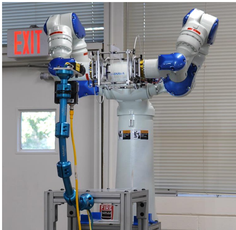
Figure 9. Robot hands operating in coordinated manipulation mode to flip the fuel cell component.
